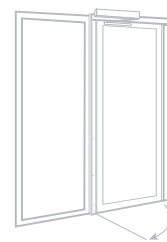
1-leaf swing door left or right opening with fixed leaves
